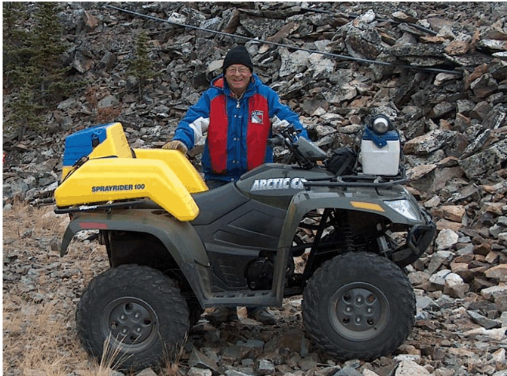
Figure A-2. Range riders used ATVs outfitted with GPS units and spray equipment to inventory rangelands and eradicate new invasions. (Photo courtesy of Liberty County, Montana.)
