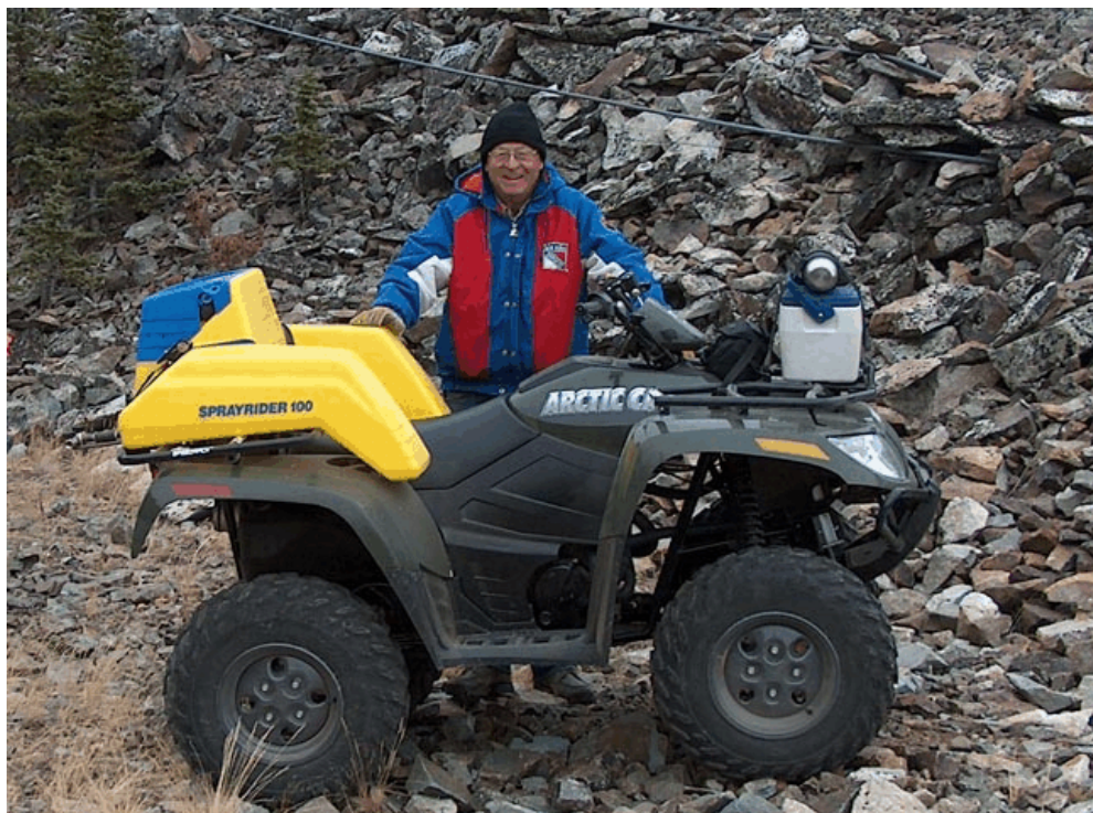
Figure F-4. Range riders used ATVs outfitted with GPS units and spray equipment to inventory rangelands and eradicate new invasions. (Photo courtesy of Liberty County.)
