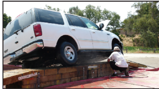
Figure 6—Cleaning ramp photo.
